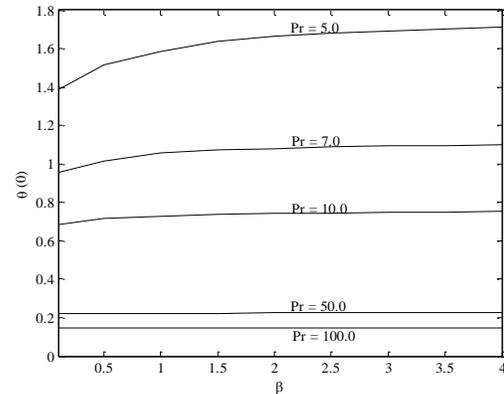
Figure 7. Variation of the wall temperature with Casson parameter when  $\gamma = 1$  for various Prandtl number.
