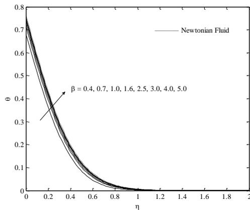
Figure 2. Variation of the temperature for various Casson parameter when  $\gamma = 1, Pr = 10$ .
