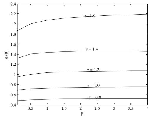
Figure 9. Variation of the wall temperature with Casson parameter when  $Pr = 10$  for various conjugate parameter.
