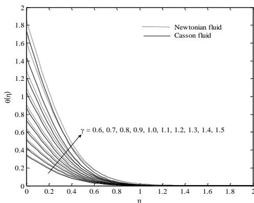
Figure 4. Variation of the temperature for various conjugate parameter when  $Pr = 10, \beta = 1.2, \beta \rightarrow \infty$ .
