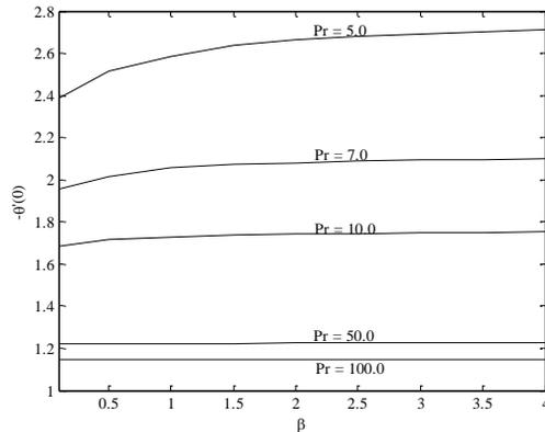
Figure 6. Variation of the wall temperature gradient with Casson parameter when  $\gamma = 1$  for various Prandtl number.
