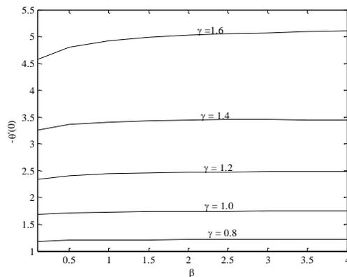
Figure 8. Variation of the wall temperature gradient with Casson parameter when  $\gamma = 1$  for various conjugate parameter.
