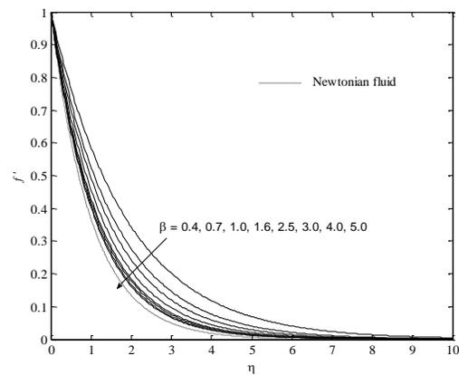
Figure 3. Variation of the velocity for various Casson parameter when  $\gamma = 1, Pr = 10$ .
